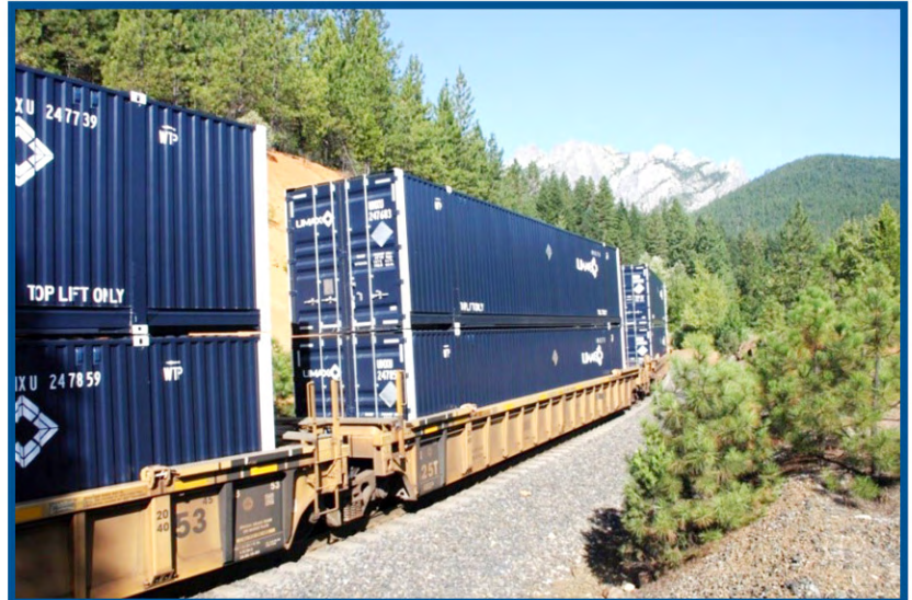
Containers are double-stacked on railcar
